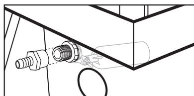
If using poly-pipe or PVC, thread the desired fitting onto the other end of the fill valve
