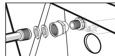
If connecting to a garden hose, thread 13mm end of the female garden hose adapter (included) to the other side of fill valve. Insert the (2) rubber gaskets into 19mm end of adapter and attach garden hose.
