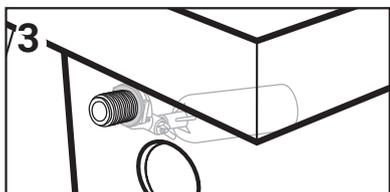
3 Insert threaded end of fill valve through the 19mm hole drilled in the side wall of unit. **Note:** Rubber washer must be located on the inside wall.
