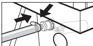
Connect 13mm irrigation line to barbed fitting and tighten with hose clamp provided in the water fill valve kit.
