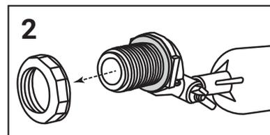
2 Remove hex nut from threaded end of fill valve, leaving only the rubber washer on.
