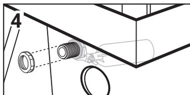
4 Tighten hex nut, securing the fill valve to the unit.
