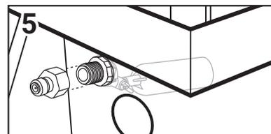
5 Attach Fitting into the Fill Valve, making sure that it's tight.
