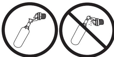
**NOTE:** Correctly orient water fill valve pointing down. Do not orient valve in the upright position.
