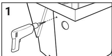
1 Drill a 19mm hole in side wall of skimmer, Pondless® Waterfall Vault, or decorative basin. Exact location for the water fill valve will be different for each unit. Fill valve location should be 25mm above the desired water level.
