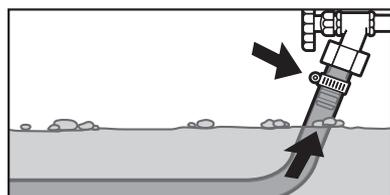
Trench 13mm poly-pipe irrigation line to water spigot and connect using a brass garden hose adaptor (not included), or connect to existing irrigation line. The irrigation line can be buried a few inches below the surface of the soil.
