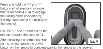
NOTE: Complete remote pairing process within 1 minute of connecting the receiver to the power source.
